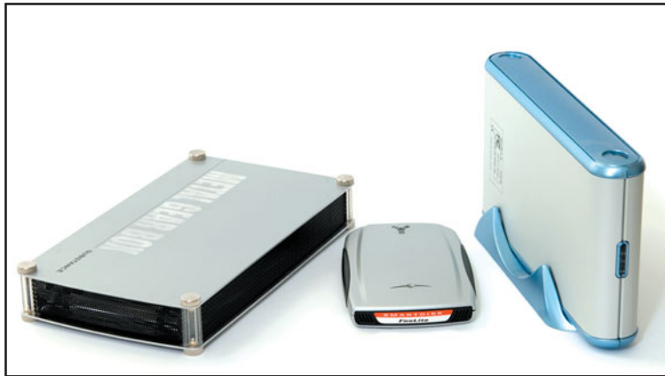
FIGURE 6.2 External USB-2 and Firewire drives make excellent storage add-ons, for backup or additional workspace. Small, 2.5" drives, like the one in the center, can take their power from the same cable that is used to connect the drive to the computer, making them ideal for taking on the road. Larger drives require separate power, but offer much larger capacities, and better price per gigabyte.
